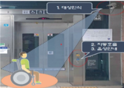
<Automatic elevator calling system>
